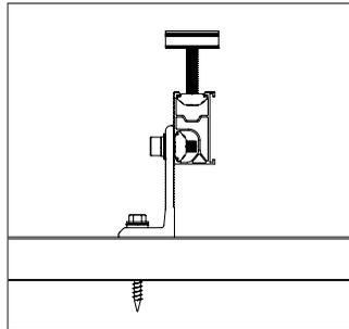
2. Place second PV module into rail, leaving a 20mm gap between modules and insert the mid clamps, slide the PV module flush against mid clamp closely, then tighten the mid clamp screw to 10 N-m using 6 mm Allen key or hex driver bit. Repeat procedure for follow mid clamps.
