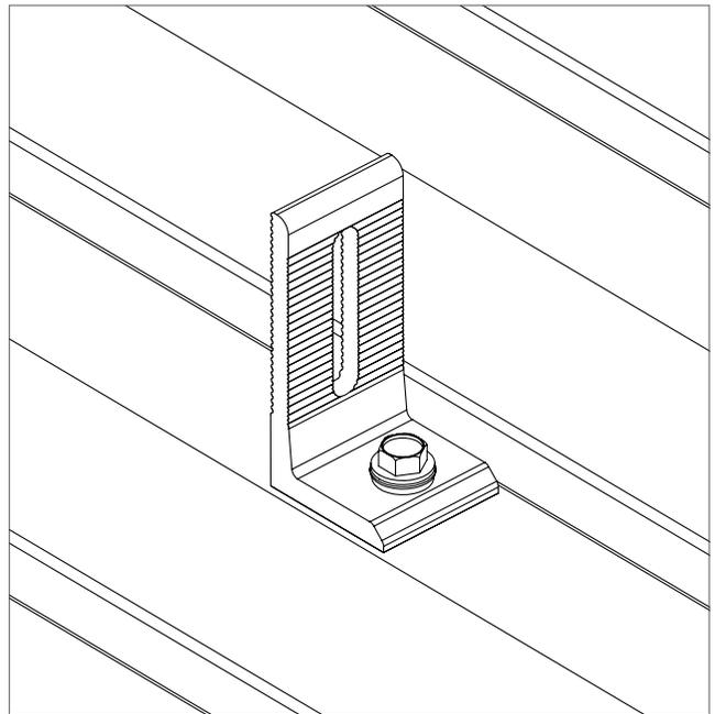
2. Fix the L foot to timber batten or steel batten/purlins with supplied screw. Fully seat.
