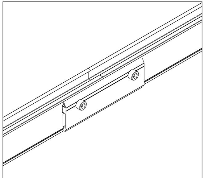
4. Connect multiple rails by using rail splice (if required per system design)
