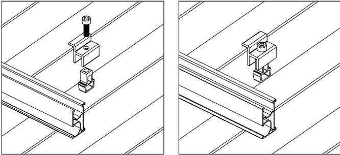
3. Place last module in position on rail with a minimal 50mm from rail end, slide end clamps onto both rails and tighten the screws to secure the PV module.
