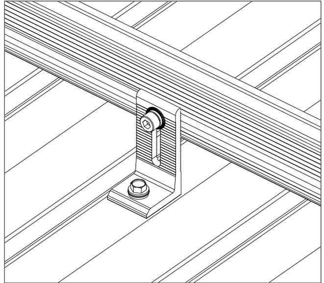
3. Connect rails to L foot to 16 N-m using a M6 Allen key or hex driver bit
